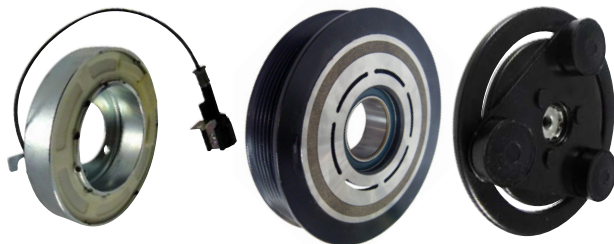
CC-6008 DKS17D NISSAN CP-66390 6GV, 134/139mmOD CH-6012 35X55X20
